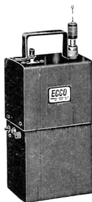
ECCO 10 METER TRANS-RECEIVER Designed for spot frequency use for emergency, CD, and net operation. Completely self-contained including batteries. Transmitter uses 20 meter crystals. Fixed frequency receiver has regenerative circuit. Base loaded 36" antenna. Carbon mike input. 1/2 watt input to final. With 5 tubes. Less mike, headphones, crystal, and batteries.
