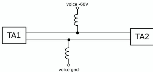
Coils are actually part of a relay. A special telephone relay with two coils and a single anchor can be used, but for now, it's okay to use two separate 24V relays. T coils pass direct current to power the phones, but resist alternating voice current and force it to go through another phone, rather than back through the power supply.
