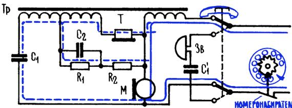
The phone does not pass direct current while on-hook, but it does pass alternating ring current. The ring capacitor value is typically  $1\mu F @ 250V$ . Some old phones have ring and voice capacitors made as a single unit, like the one shown here, but they are two separate capacitors anyway. So we need to apply al-
