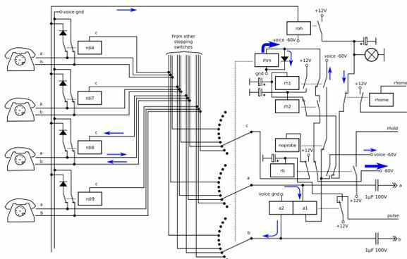
I'm going to show you a more complicated design, one that I've built. It has just two rotating switches, so only one pair of telephones may use the connection kit, and other telephones must wait their turn. Up to ten phones may be used total. There is no dial tone circuit, as that would require an additional coil on the A1-A2 relay.
