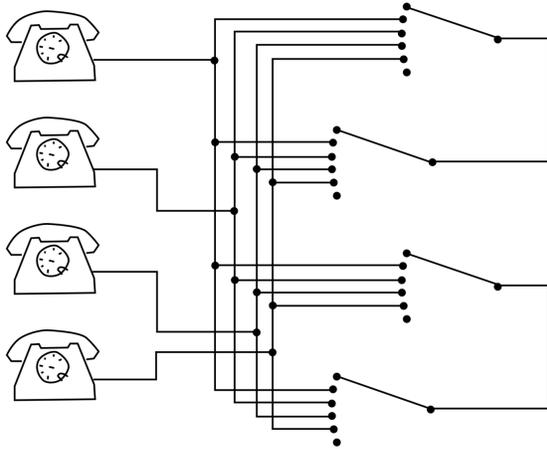
Switch operation may be driven by pulses coming from the phone, which is slow, or it may be free switching, where the switch quickly steps itself until it finds the right position.
