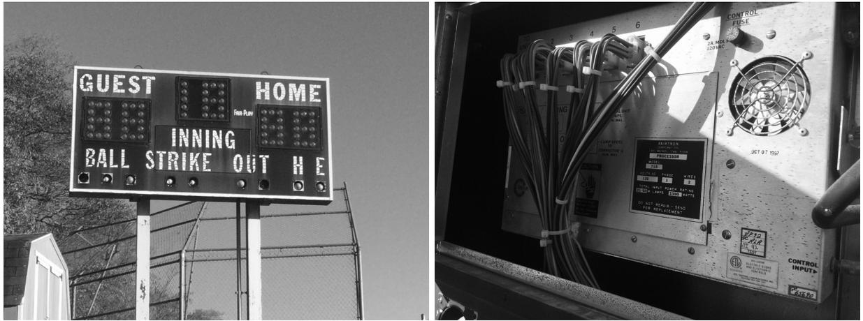
Figure 2: FairPlay 710 scoreboard and internal processor box.
