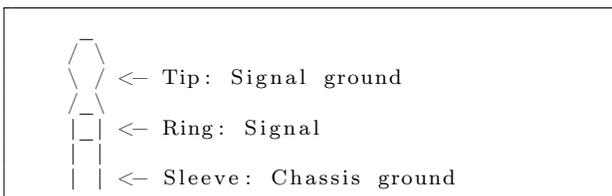
The FairPlay signal uses RS-232 signal levels ( $\pm 5V$ ), but uses a proprietary protocol. In RS-232, each bit takes the same amount of time, with a 1 being a logical high (+5V) and a 0 being a logical low (-5V). The length of each bit is determined by chosen baud rate. In the FairPlay protocol each symbol contains both a high part and low part, and the difference between a 1 and a 0 is the length of the high part. Each symbol is 30 microseconds long,
