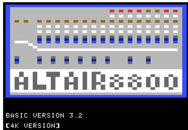
I could now create and run a program in an interpreted language created by a program running on a virtual 8080 processor, emulated by another program running on a 6502 processor.
