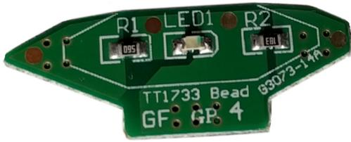
The bracelet itself has slots on the sides to hold six Z-Crystals and one on the top that has the signature giant Z around it. The slot on the top has three pogo pins, which connect to pads on a Z-Crystal. The center of these is GND, with one pin being used to light the LED through a series resistor (R1, 56  $\Omega$ ) and the other pin being used to sense an identity resistor (R2, 18 k $\Omega$  for green).
