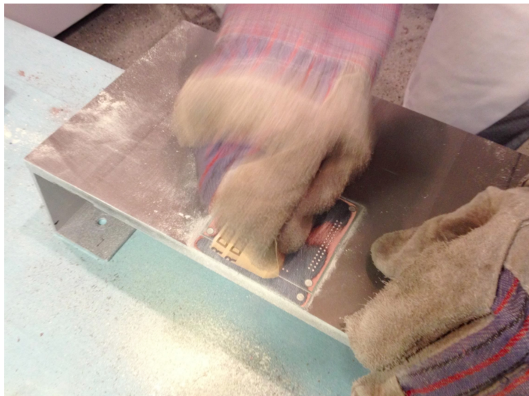
Figure 20: Sandpaper at work. You can see the copper of inner layer 2 starting to peek out from underneath the top substrate.
