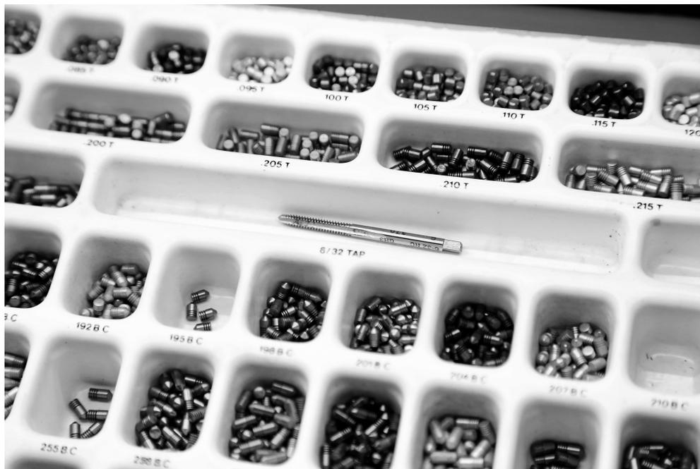
If you have the knowledge of even basic lock field-stripping, it is quite possible to upgrade a pin tumbler lock using this technique for very little cost. The LAB company's S-pins are available for less than a dime each<sup>13</sup> and hardware tool suppliers sell both the 6/32" tap and a suitable tap handle for four dollars apiece.
