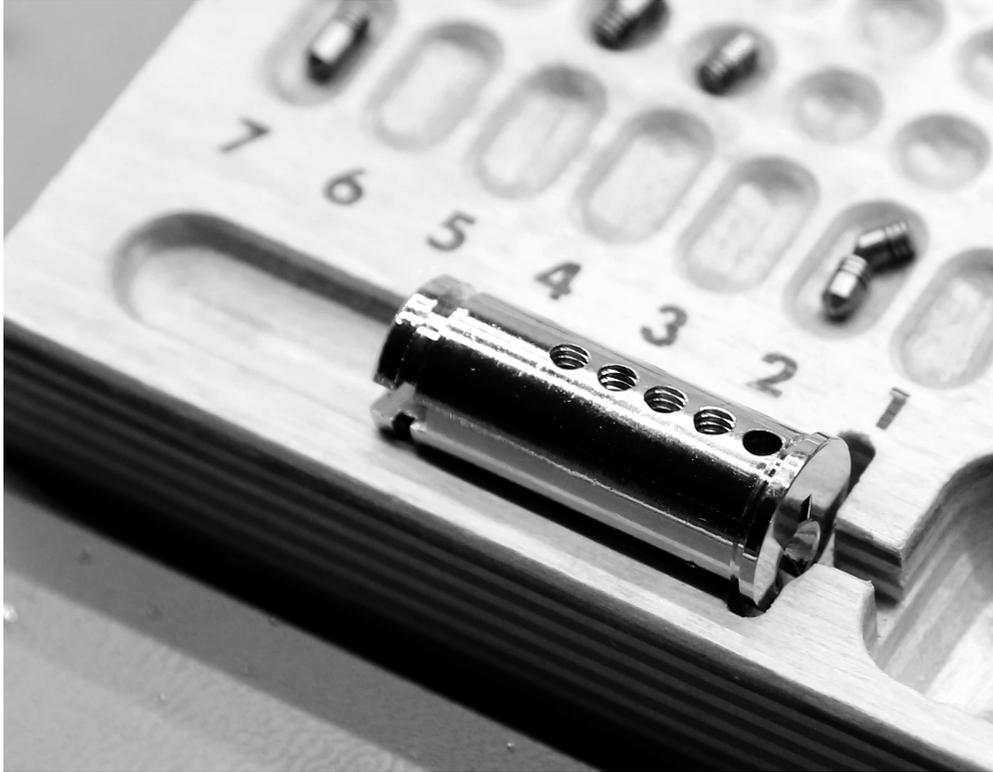
By cutting these threads into the pin chambers, a much greater degree of friction and positive lock-up between the pins and the plug can be achieved. If there is turning pressure on the plug—as there is with a lockpicking attack—and any attempt to push the pin stacks is made, the serrations will bite together. This is remarkably robust for a number of reasons:
